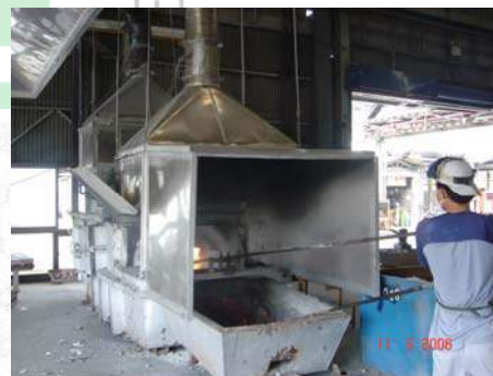
(a) Enclosures - contain contaminants released inside the hood
